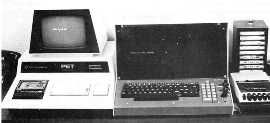
Photo 3. Now-defunct Sphere, right, is very similar to PET, left. Note the combined keyboard, TV, CPU, integral dual cassette controls and number pad. PET's cassette is built in.
