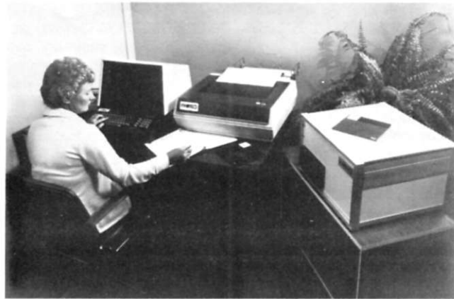
The CRT, printer and disk that make up the Infotecs complete system. The 6100 CPU and memory are in the disk unit.
