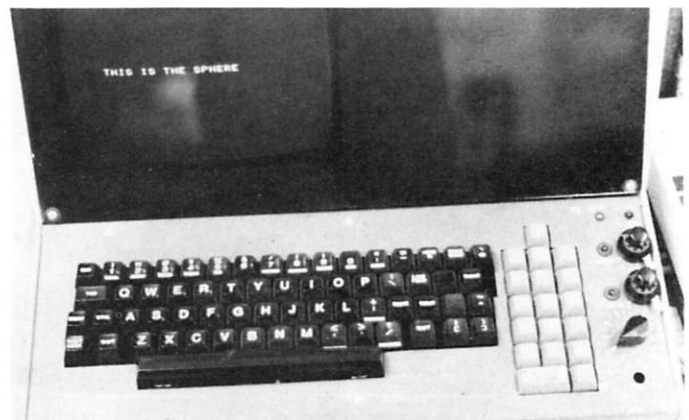
Photo 5. My Sphere's original alpha keyboard was replaced as shown. Note pasted editing and control labels on fronts of keys. Specialized timing controls at far left are not standard.
