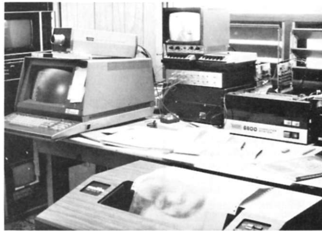
Photo 1. The Micro Works system; TV camera on the left, SWTP system; Malibu Design Group printer.
